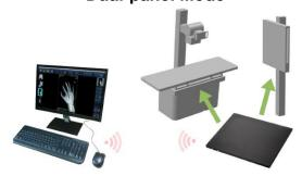
2 Flat Panel Detectors are used with only one console by our DX Easy Imaging Software.
