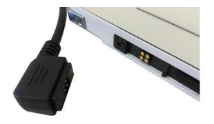
With the flexible design of our FPD it is possible to switch between different operation modes by plug and play. Simply unplug the TCP/IP Data cable to use the panel wireless and vice versa without a need of a new configuration of the device. A magnetic connector for the power plug ensures easy online switching between line operation and battery operation. This enables a fast change between fixed place and mobile mode operation of the panel.
